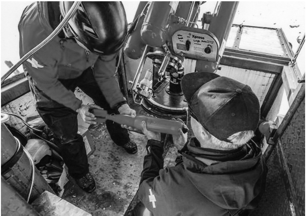
This is the “avalauncher” machine used by the ski patrol at Turoa to bomb avalanche prone slopes after a heavy snowfall. The cannon uses compressed nitrogen gas to fire missiles up to 1.4km where they explode on impact with the surface of the snow. Photos: RAL.
